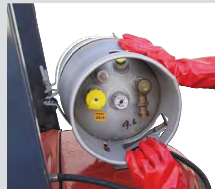
4. WATCH FOR ESCAPING GAS FROM FUEL LINE
