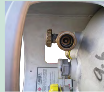
2. ENSURE O-RINGS IN FORKLIFT VALVE ARE IN GOOD CONDITION. SEE ADDITIONAL SAFETY TIPS SEC-
