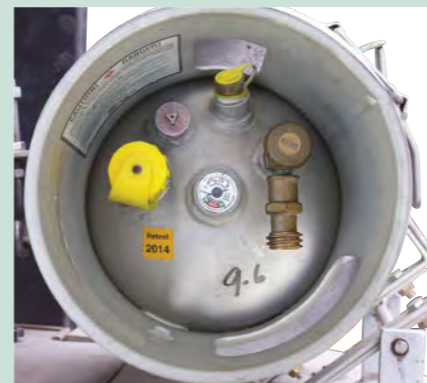
4. ENSURE TAP IS TURNED OFF ON GAS CYLINDER
