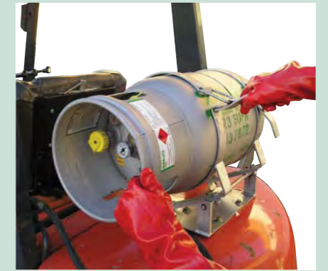
3. ENSURE PRESSURE RELIEF VALVE IS AT THE TOP AND THEN SECURE BRACKET HOLDERS
