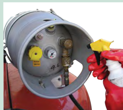
7. SPRAY CYLINDER WITH SOAPY WATER TO ENSURE THERE IS NO LEAKAGE
